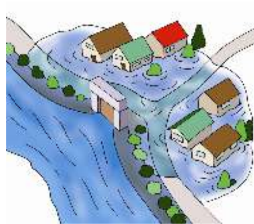
Figure 2.36 Internal Flooding Situation
